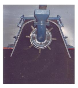
The shape and size of the parts determine the number of turbines used in a machine. Power of the turbine motor is based on degree of cleaning needed and throughout speed of the material.
