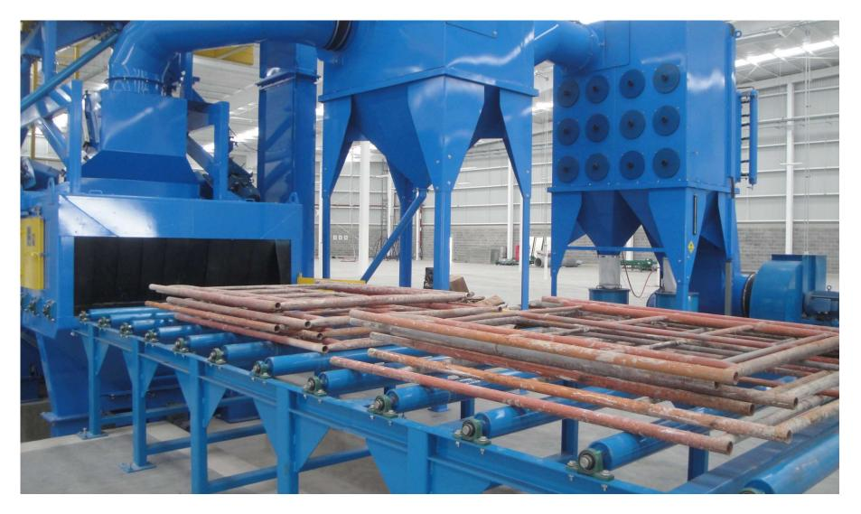
Cym Materiales SA manufactures continuous flow equipment for **shot blasting welded scaffolding, metal formwork, planks, reins, walkways, ladders, props and related accessories** according to the needs of each customer.
